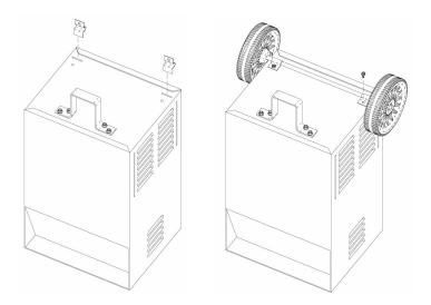
**9.5** Attach the Handle: If the charger came with a plastic grip, slide that onto the handle until it is centered at the top. Turn the charger right side up onto its foot and wheels. Align the handle so the screw holes are aligned with the screw holes on the upper back corners of the charger. Attach the handle using the four Phillips head screws provided.
